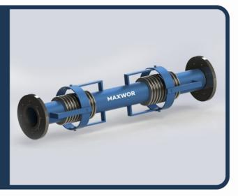
Gimbal type Expansion Joints are absorbed axial movements, lateral deviations and angular rotation with containing two bellows. Since it is an FM approved product in fire circuits, it has an absolute use in dilatation passages. Design and production are made according to "EJMA" standards. Pressure and temperature values comply with DIN2401 standards. It has the capability of damping or absorbing all kinds of movements thanks to its bellows and universal joints on its double side.
