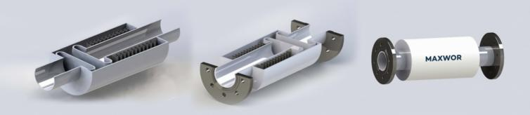
A heating pipeline system at 90/70°C causes approximately 3 mm of movement for each floor of the buildings. The expansion in the column line of a 7-storey(21 meters) building can be taken with the elbows in the vent and main line collection. The pipe expansion joint, which must be used in the column lines of buildings higher than 7 floors, should be used at most every 30 meters(every 10-storey).
