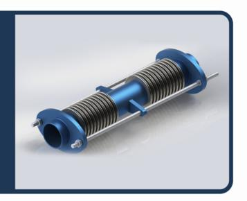
Universal tied expansion joints are made up of two bellows connected each other by an intermediate pipe and a system of tie rods able to withstand the thrust resulted of the internal pressure. Universal tied expansion joints are absorbed 50, 100, 150 and 200 mm lateral movements as standard, also special productions are possible for other desired expansion values. In this type of compensators, the part is stabilized by using control rods.
