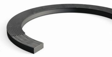
particularly suitable for applications where high temperatures, pressures and fluctuating conditions are encountered. Non-metallic cover layers ensure that flanges are not damaged, even at extreme loads, and that they provide excellent sealing properties when supported by the grooved metallic gasket. The grooved gasket can be used as an alternative for applications associated with jacketed gaskets (for heat exchangers, vessels and reactors and various flanged connections).
