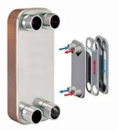
Brazed plate heat exchangers, which are different from gasketed plate heat exchangers, are used where sealing is important. They are equipment that is sealed at high temperature, under vacuum, using copper or nickel materials.
