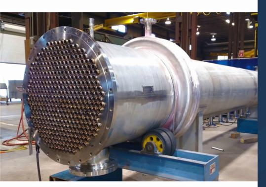
Necessary information to design a shell and tube heat exchanger; flow rate, temperature and physical properties of fluids. Besides, other data that may be important depending on the application are the inlet pressure, maximum acceptable pressure drop and flow rate.
